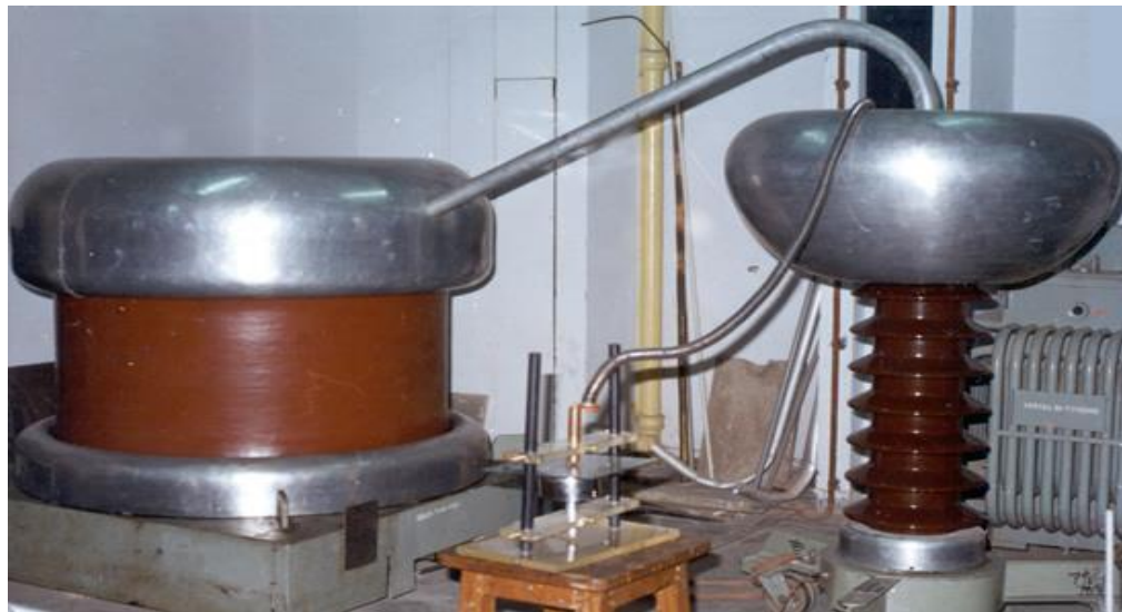
Fig. 4 A PB free 100 kV Transformer and 1.1 nF Coupling Capacitor setup in HV Laboratory at IIT Kanpur
