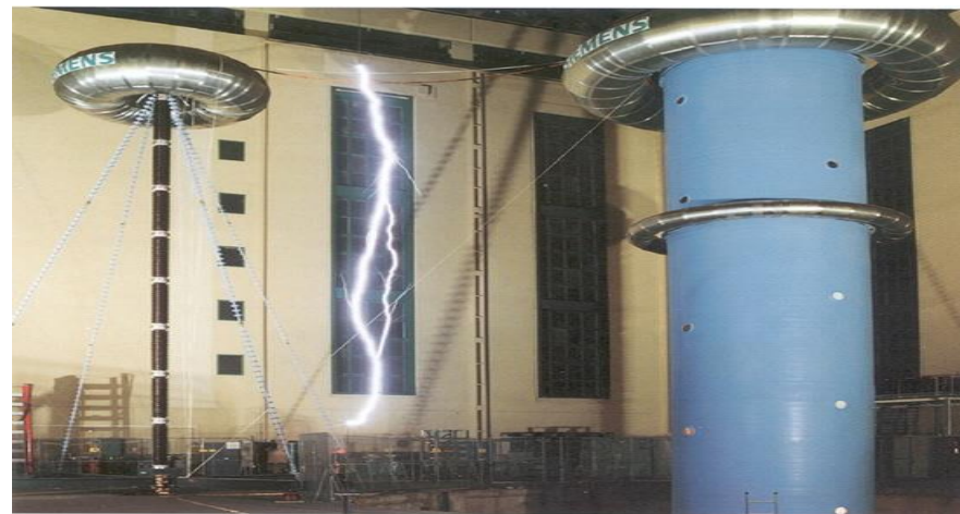
Fig. 5. Damped capacitive-resistive voltage divider (on the left) the measurement of 4.5 MV impulse voltage (generator on right), courtesy Siemens (now High Volt), Dresden, Germany
