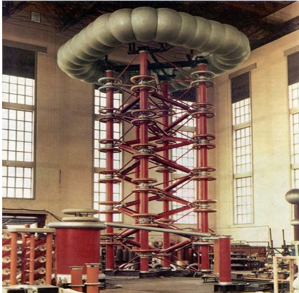
Fig. 13 A 2000 kV HVDC test set, courtesy TüR Dresden, Germany
