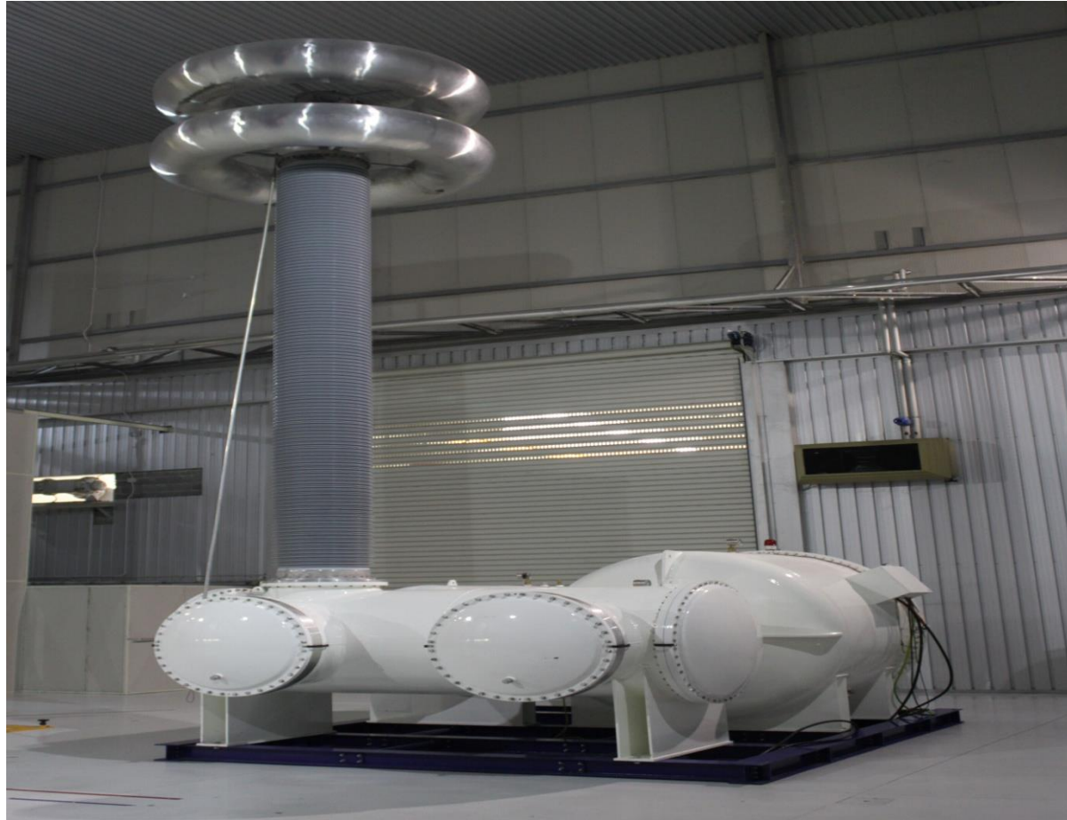
Fig. 2 An SF 6 gas filled 1000 kV, 0.6 A, single unit ac power frequency test transformer, courtesy Himalayal Test Systems, China.
