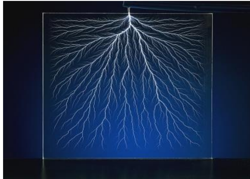
Fig. 19 Development of Treeing Process in Epoxy Resin, used with permission from Bert Hickman, Stoneridge Engineering, LLC, http://capturedlightning.com , Hickman [6.6].
